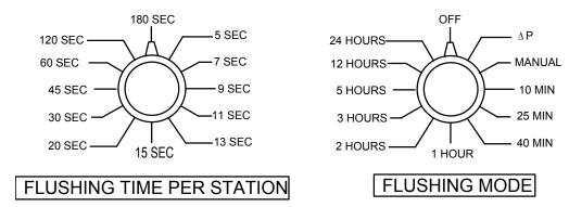
• The FLUSHING TIME PER STATION / FILTER switch must be set before the system is switched on. The time can be obtained from the following table:
