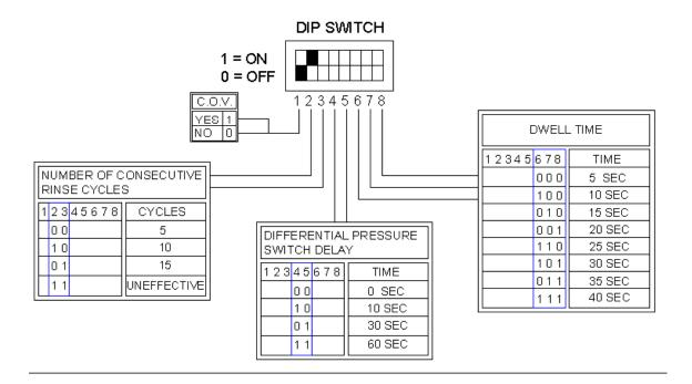
**COV Presence:** Position 1 of the DIP Switch tells the controller if a Controlled Outlet Valve (COV) is present. The up position (ON) indicates that a COV is present and the valve's solenoid is connected to the last available output. At the start of a rinse cycle, the COV output is energized first, then after a fixed 16 second delay, the filter's solenoid is energized. The COV output stays energized until the filter(s) rinse cycle is complete.
