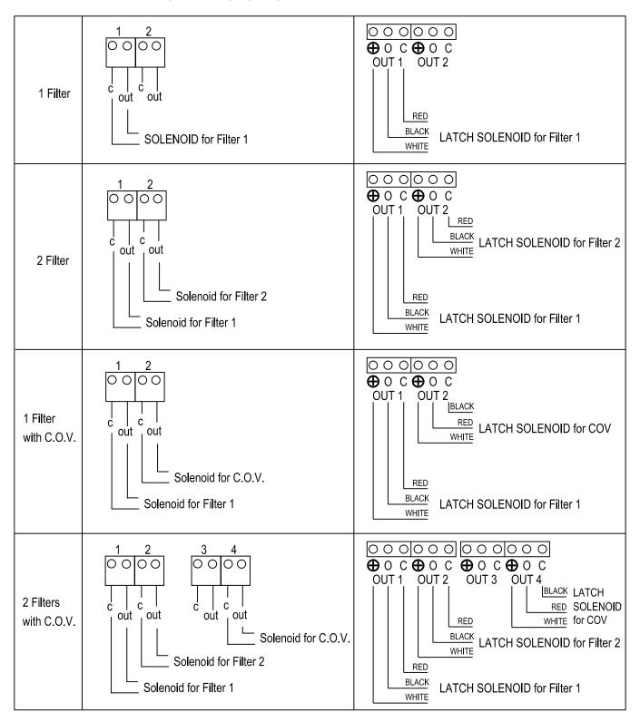
NOTE: FILTER SOLENOIDS ARE CONNECTED AS Normally Closed & A COV SOLENOID IS CONNECTED AS Normally Open
