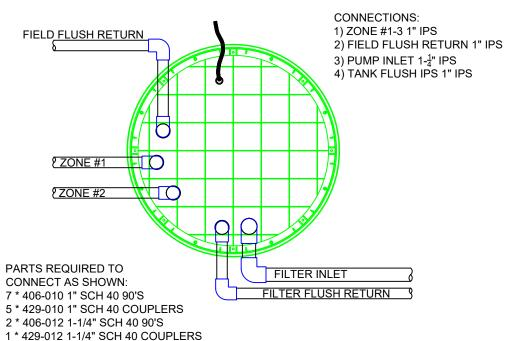
TYPICAL INSTALLATION AND PIPING DETAIL
